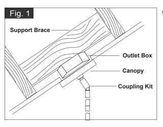
Angled mounting recommended for a vaulted or angled ceiling. (See Fig.1)
