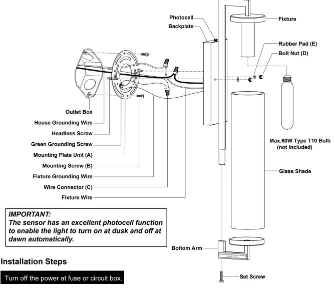
1. Unscrew the two bolt nuts (D), remove the two rubber pads (E) and the mounting plate unit (A) from the backplate.
