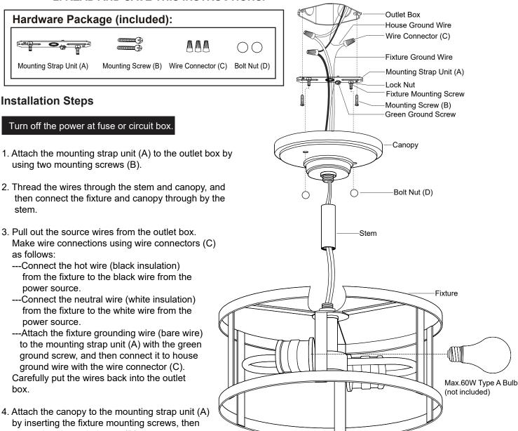
secure it with two bolt nuts (D).
