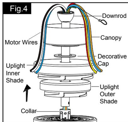
Thread the motor wires through the upright inner shade, upright outer shade, decorative cap (Making sure the smooth side of decorative cap is facing downward.), canopy and downrod.
