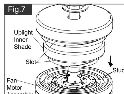
Secure the upright inner shade onto fan motor assembly by aligning studs and slots, and turn clockwise until it is locked in place.
