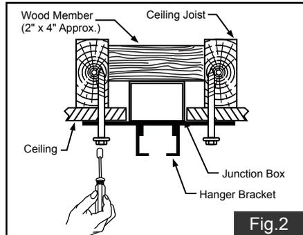
Tighten the hanger bracket to the outlet box with two mounting screws. **(Make sure the outlet box is securely installed so that it will be able to support at least the fan weight.)** Attach the safety cable hook to the ceiling with the drywall screw and washer, and make sure the safety cable hook is covered by the fan canopy.
