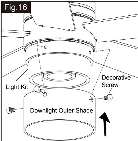
Align and engage the hole of downlight outer shade to the side hole of light kit, then secure them together with the decorative screws which provided in assembly kit by your hand.
