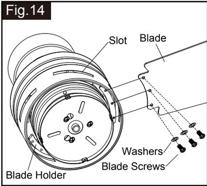
Insert the blade into blade holder according slot then tighten blade to blade holder by using blade screws and washers. Repeat to other blades.
