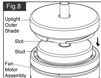
Secure the upright outer shade onto fan motor assembly by aligning studs and slots, and turn clockwise until it is locked in place.
