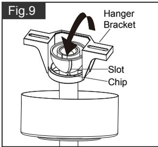
Hang the fan on hanger bracket, and make sure the slot of hanger ball is snapped into the chip of hanger bracket exactly.
