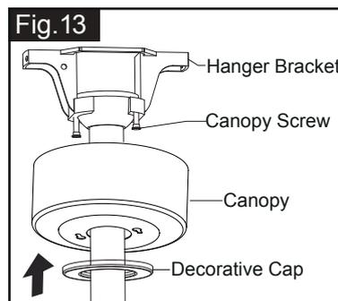
Slide the canopy up to ceiling and over the two canopy screw on hanger bracket. Rotate canopy clockwise, next, while holding the canopy with one hand, slide the decorative cap over the screws and rotate clockwise until tight.
