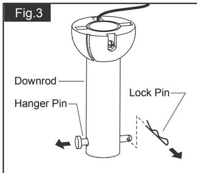
Remove the lock pin from hanger pin and remove the hanger pin from the downrod.
