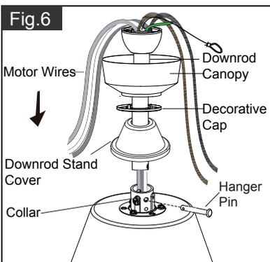
Insert the downrod into the collar. Slide hanger pin through holes of collar and downrod.
