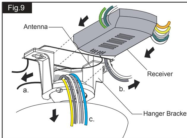
Move ground wires (a), outlet box wires (b), and motor wires (c) way from the center of the hanger bracket as shown. Thread the antenna through the hanger bracket first, then thread the receiver through the hanger bracket until it is placed in the center. Finally, cut motor wires (c) to length needed for connections.
