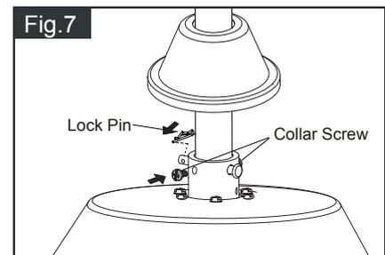
Insert the two collar screws into the collar until tight. Slide lock pin into hanger pin until it is locked into position.
