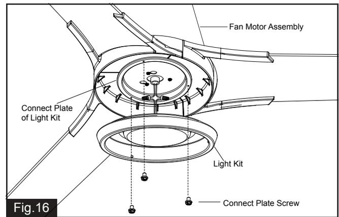
Remove three connect plate screws from connect plate of light kit first (for later use). Then connect the white (neutral) wire from the light kit to white (neutral) wire from fan motor assembly with a wire connector; connect the black (hot) wire from light kit to blue (hot) wire from fan motor assembly with a wire connector. Carefully put the wires into the connect plate of light kit, then attach the light kit onto the connect plate of light kit with the connect plate screws.
