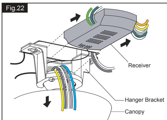
Unscrew the canopy. Remove the wire connectors from the fan to ceiling wire connection. The receiver should be removed from the hanger bracket. (See Fig.22)
