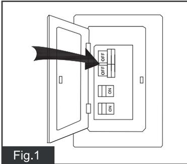
Turn OFF the electric circuit at the main fuse fuse or circuit breaker box.
