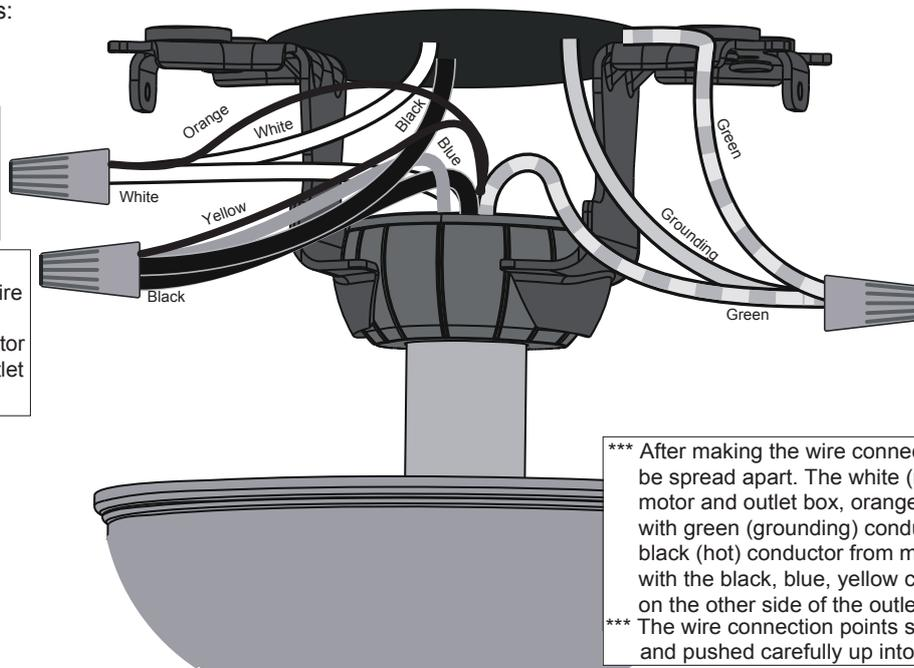
\*\*\* After making the wire connections, the wires should be spread apart. The white (neutral) conductor from motor and outlet box, orange conductor from motor with green (grounding) conductor on one side; the black (hot) conductor from motor and outlet box with the black, blue, yellow conductor from motor on the other side of the outlet box.
