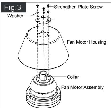
Align and engage the fan motor housing and strengthen plate to the fan motor assembly. Then secure the strengthen plate to the fan motor housing with washes and strengthen plate screws.
