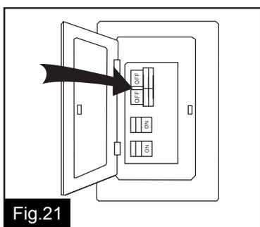
Turn OFF the electric circuit at the main fuse or circuit breaker box. (See Fig.21)
