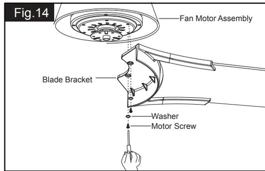
Remove the motor screws and washers from the fan motor assembly. Secure blade brackets to the motor with washers and motor screws.
