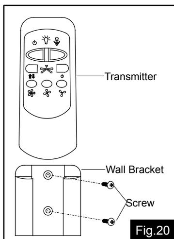
Install the transmitter wall bracket on the wall with two screws and place transmitter in it carefully.
