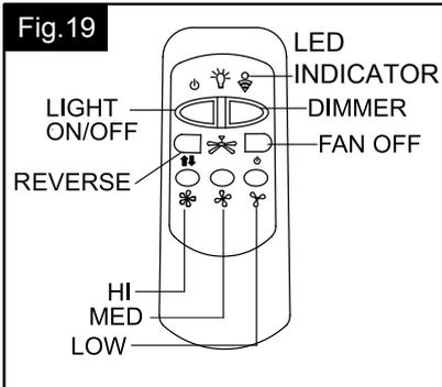
Install the battery (9V, included) into the transmitter.
