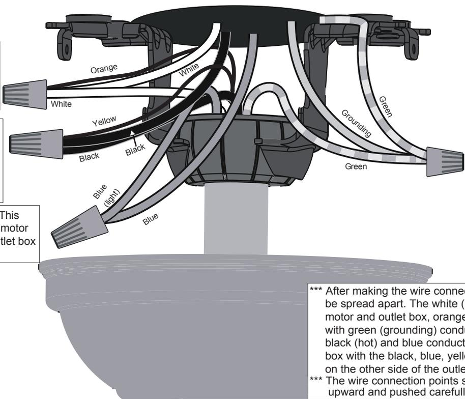
\*\*\* After making the wire connections, the wires should be spread apart. The white (neutral) conductor from motor and outlet box, orange conductor from motor with green (grounding) conductor on one side; the black (hot) and blue conductor from motor and outlet box with the black, blue, yellow conductor from motor on the other side of the outlet box.
