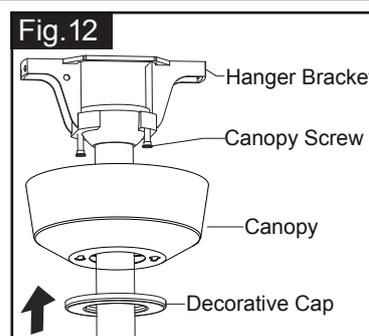
Slide the canopy up to ceiling and over the two canopy screws on hanger bracket. Rotate canopy clockwise, next, while holding the canopy with one hand, slide the decorative cap over the screws and rotate clockwise until tight.
