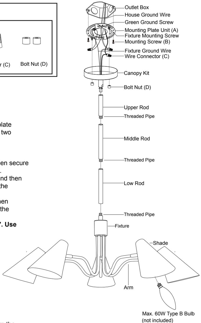
5. Attach the fixture onto the mounting plate unit (A) and tighten it with two bolt nuts (D).
