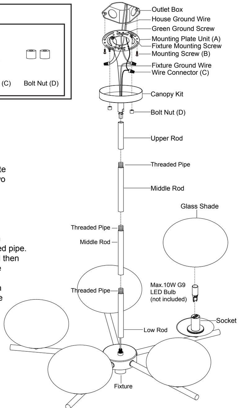
6. Attach the fixture onto the mounting strap unit (A) and tighten it with two bolt nuts (D).
