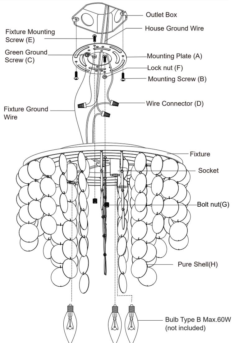
6. Install bulbs (not included). See relamping label at socket area or packaging for maximum allowed wattage.
