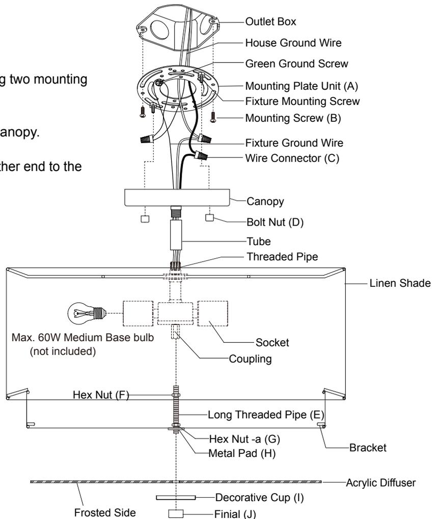
7. Pull out the source wires from the outlet box. Make wire connections using wire connectors (C) as follows:
