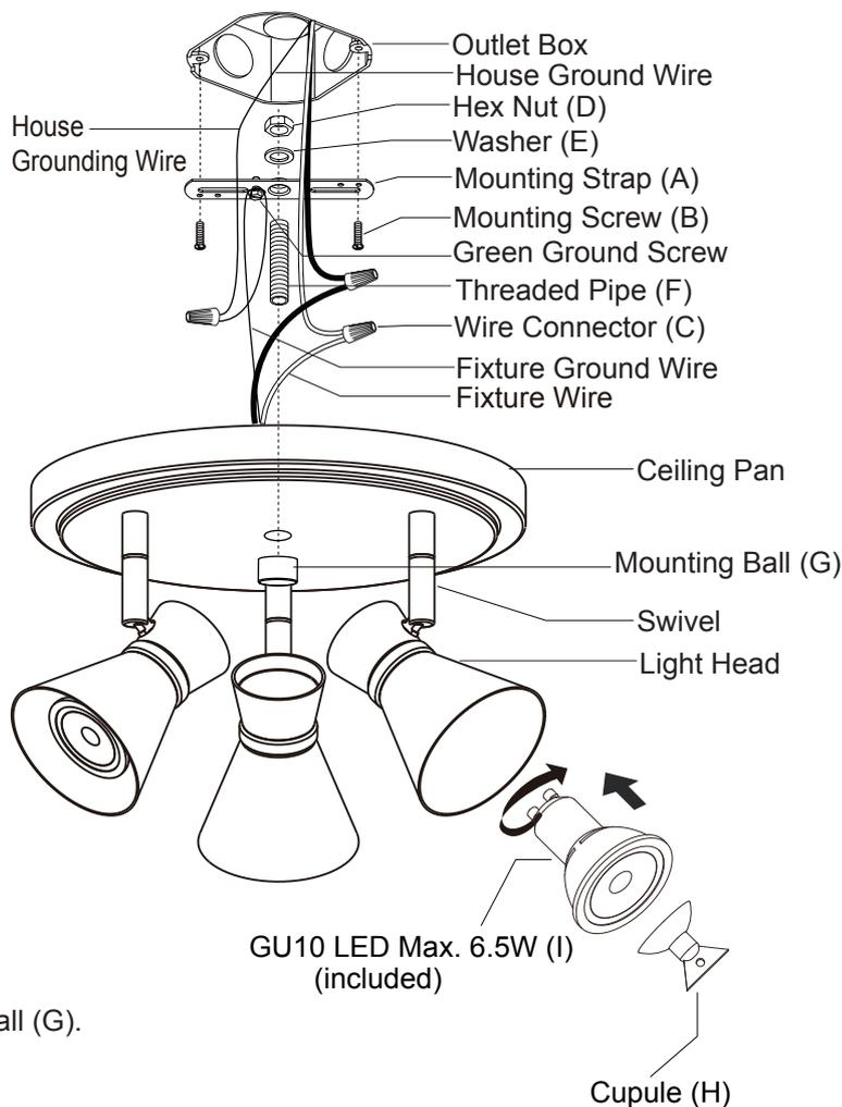
5. Attach the cupule (H) to the top surface of the bulb lens. Insert the bulb (I) into the socket using the cupule (H). Twist bulb to lock pins in place. Remove the cupule (H) from the bulb lens by pulling the knob of the cupule (H).
