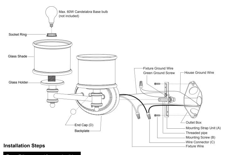
Turn off the power at fuse or circuit box.
