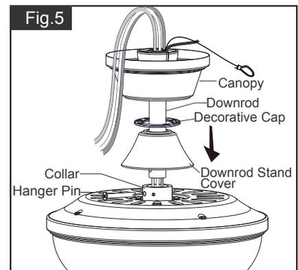
Loosen the collar screws out part way. Insert the downrod into the collar. Slide hanger pin through holes of collar and downrod.
