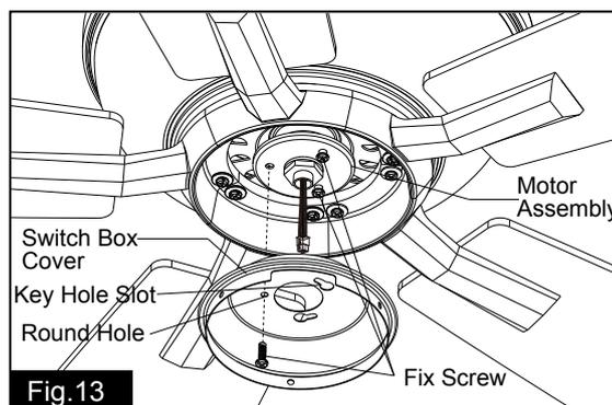
Remove one fix screw (for later use), and loosen the other two fix screws. Thread the wire through the switch box cover, and then push the switch box cover upwards by inserting the other two fix screw heads into key hole slots, rotate the switch box cover till the round hole in switch box cover aligns the hole in motor assembly, finally, secure the switch box cover to motor assembly with previous fix screw and tighten the other two fix screws.
