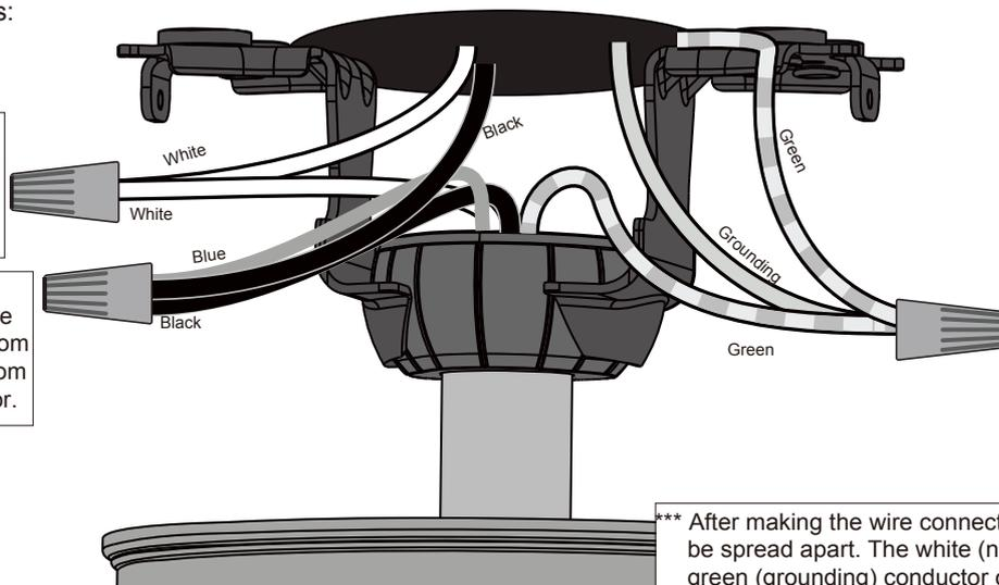
Connect three ground wires (Green or bare copper) coming from outlet box, downrod and hanging bracket with a wire connector.
