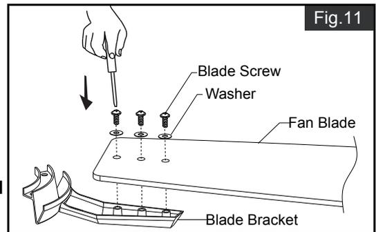
Tighten fan blades to blade brackets by using washers and blade screws.
