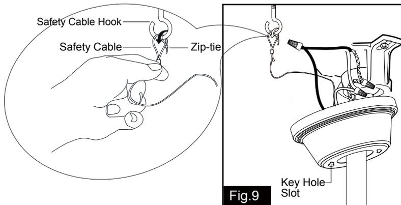
Hang the safety cable into the safety cable hook, tighten the safety cable to the safety cable hook by using the zip-tie.
