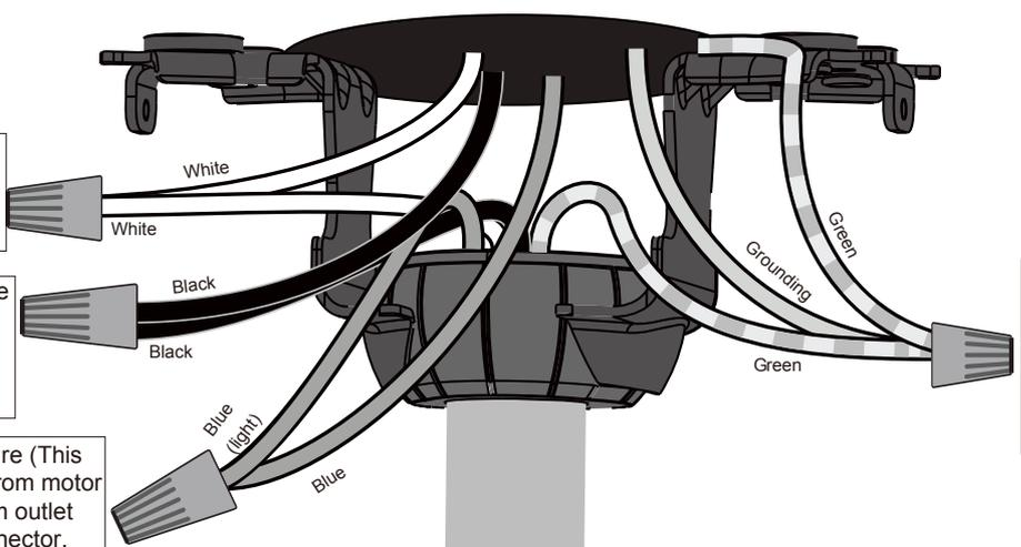
Connect three ground wires (Green or bare copper) coming from outlet box, downrod and hanging bracket with a wire connector.
