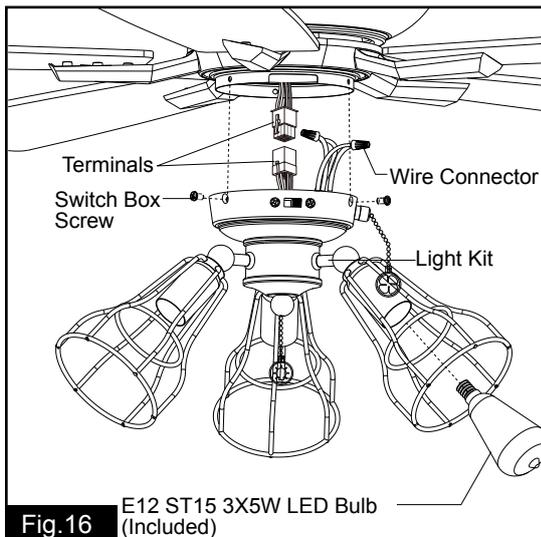
Fig. 16 E12 ST15 3X5W LED Bulb (Included)
