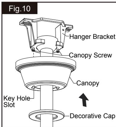
Slide the canopy up to ceiling and over the two canopy screws on hanger bracket. Rotate canopy clockwise, next, while holding the canopy with one hand, slide the decorative cap over the screws and rotate clockwise until tight. **Note: Adjust the canopy screws as necessary until the canopy and canopy cover are snug.**
