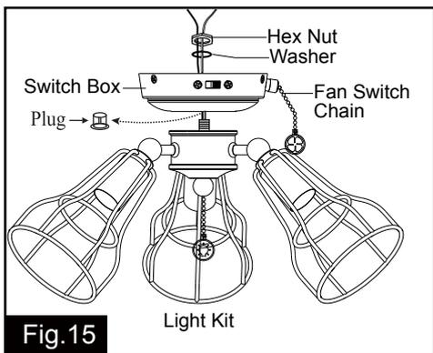
Remove the plug from the switch box. Remove the nut and lock washer from light kit. Attach the light kit to the switch box by threading the light kit wires (black and white) and the threaded pipe through the hole of switch box and then secure them onto the switch box with nut and lock washer.
