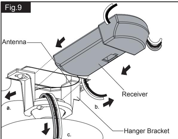
Move ground wires (a), outlet box wires (b), and motor wires (c) away from the center of the hanger bracket. Then slide receiver through hanger bracket as shown. Antenna end first, until it is placed in the center. Finally, cut motor wires (c) to length needed for connections.
