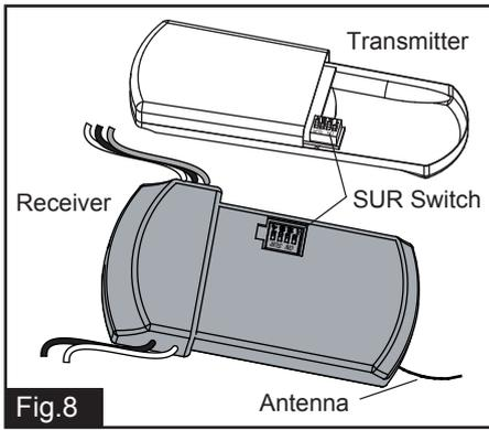
Both the transmitter and receiver have a 4-key unit code on each SUR Switch (Fig.8) and by default, all keys are pre-set to the "off" position. This means that the transmitter and receiver are already paired together. However, if you have multiple fans and remote controls and want to avoid interference between them, you can "pair" other transmitters and receivers together by adjusting the SUR switches, so the same numbered keys are in the "ON" position on both (Fig.8a).
