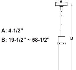
Fig. 2 Support Brace Outlet Box Canopy Coupling Kit
