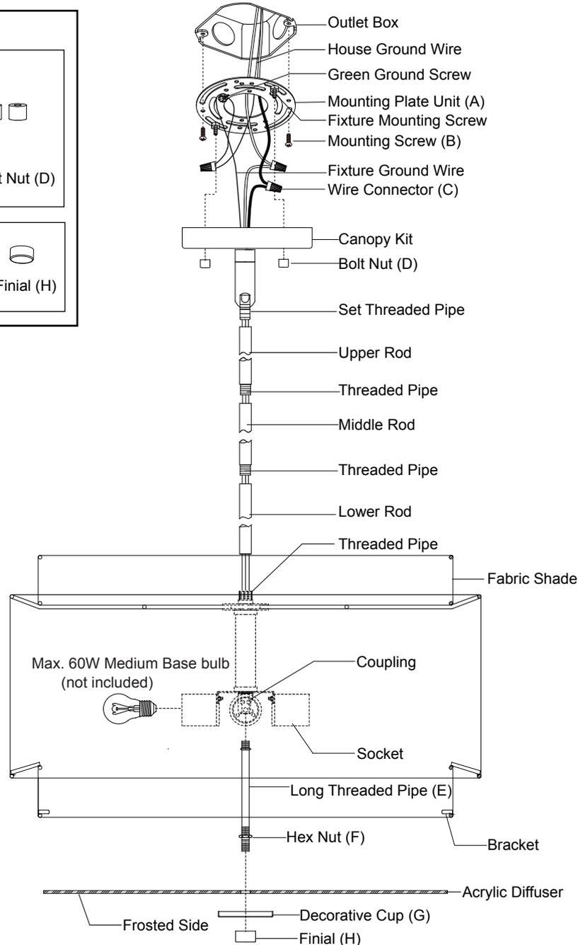
7. Pull out the source wires from the outlet box. Make wire connections using wire connectors (C) as follows:
