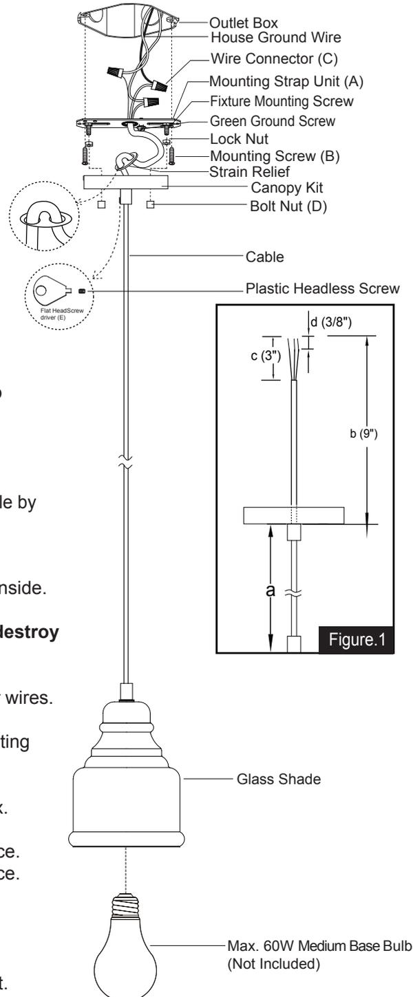
9. Attach the fixture canopy to the mounting strap unit (A) by inserting the screws, and secure it with two bolt nuts (D).
