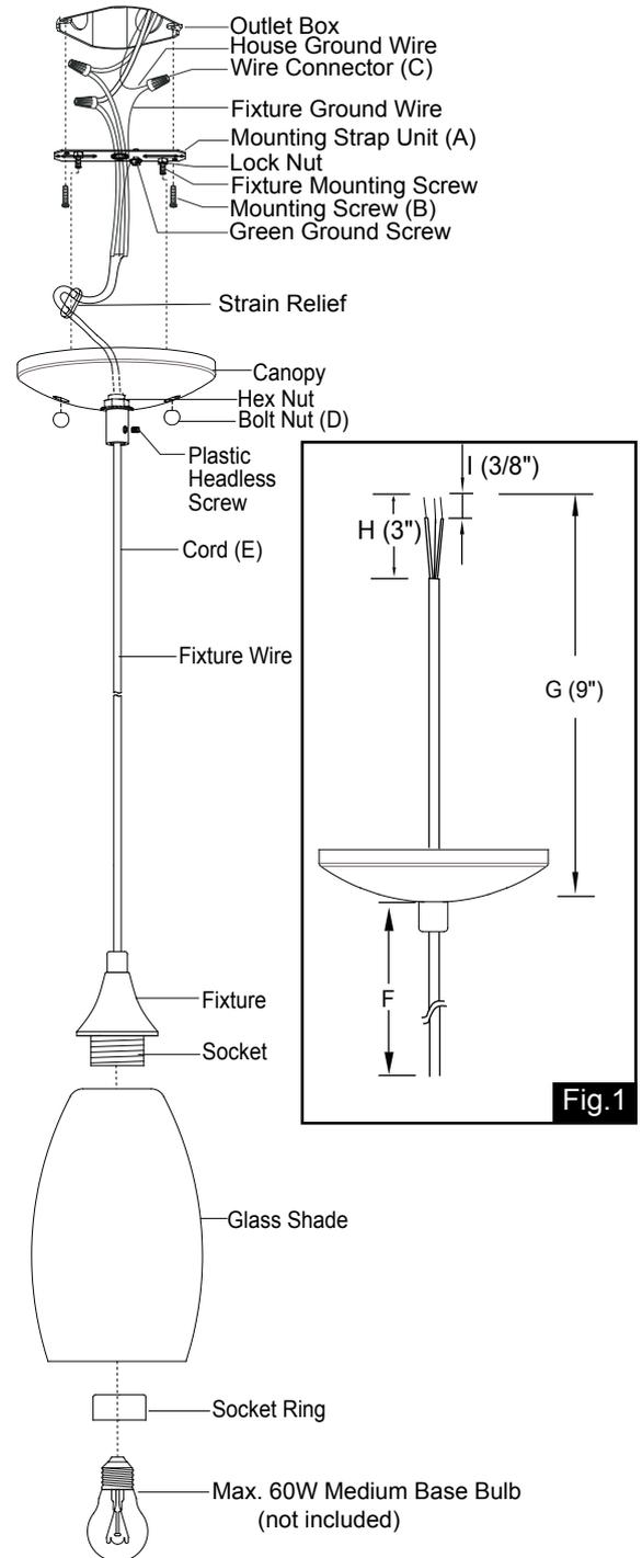
10. Fastening cord by screwing plastic headless screw, using flat head screwdriver (not included).
