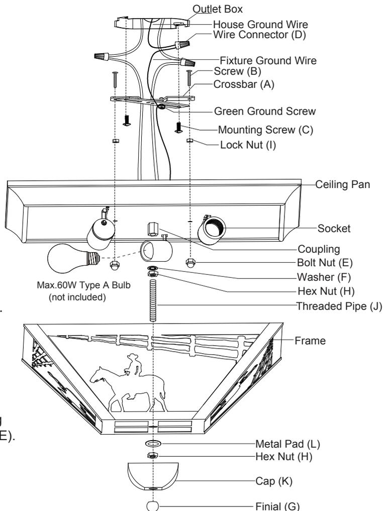
5. Install 3 x 60W max. medium base bulbs (not included). See relamping label at socket area or packaging for maximum wattage allowed.
