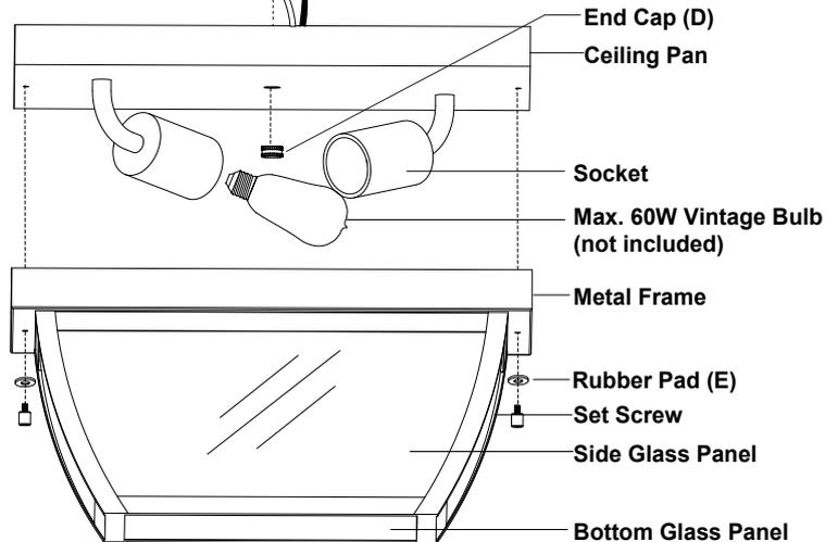
3. Attach the ceiling pan to the mounting strap unit (A) by inserting threaded pipe into the center holes of the ceiling pan and screw it with the end cap (D).
