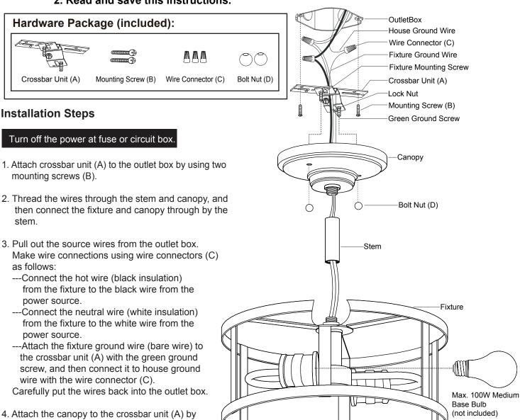
inserting the fixture mounting screws, then secure it with two bolt nuts (D).
